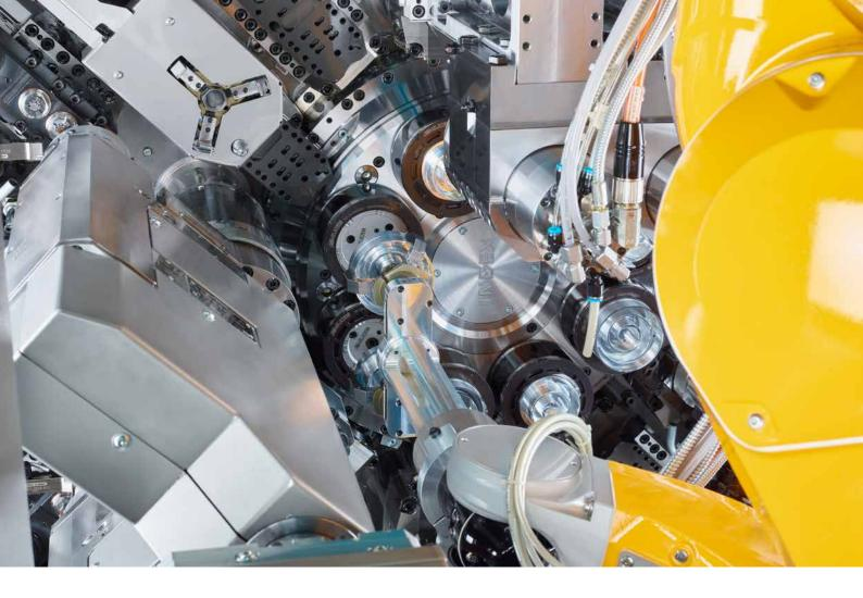
Our INDEX MS40-8 CNC multi-spindle lathe is extremely versatile. One good example thereof is the scroll machining system we developed. This variant can create precision in the µm range. It can hardly be surpassed in terms of costeffectiveness when it comes to large-scale production.
