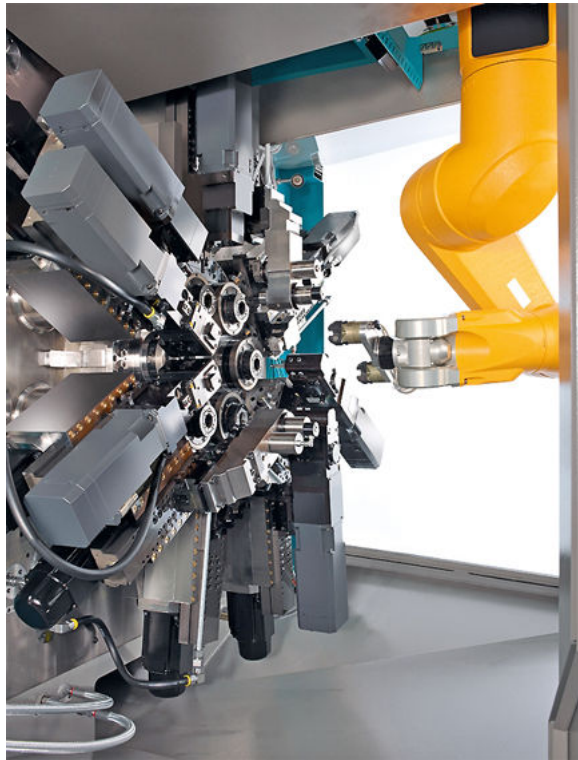
Example: MS with robot arm (Stäubli)
