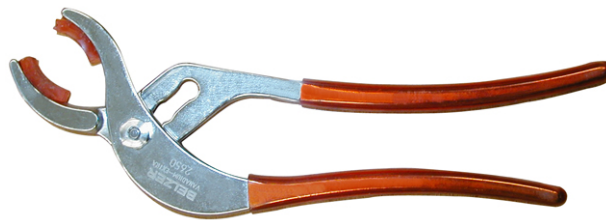
Example: Special pliers for tightening power and encoder connections on the motors
